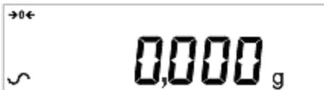
A stable sign ~ is shown when the balance is instable condition. It will turn off if the balance is not stable. Exact zero is shown when the “→0←” symbol is on to the left of the display area.
