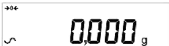
The display will show zero reading along with the zero symbol “→0←” and the weighing unit last used. If automatic time calibration is enabled the balance will calibrate 15 minutes after power up or again after the pre-set time interval.
