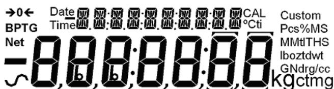
When the balance is first switched on, it will display the balance serial number (if set), software revision, model capacity and then all segments on the display will be shown. Overall the time taken is usually 5 -10 seconds.
